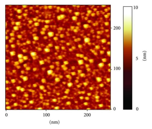
Figure 5 AFM images of the silver nanoparticles prepared by AgNO3 and lecithin
