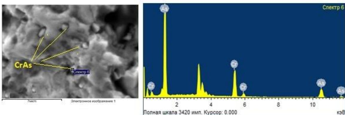
Figure 2. SEM micrographs of InAs-CrAs showing cross sections of the samples along the lateral directions of the CrAs phase.
