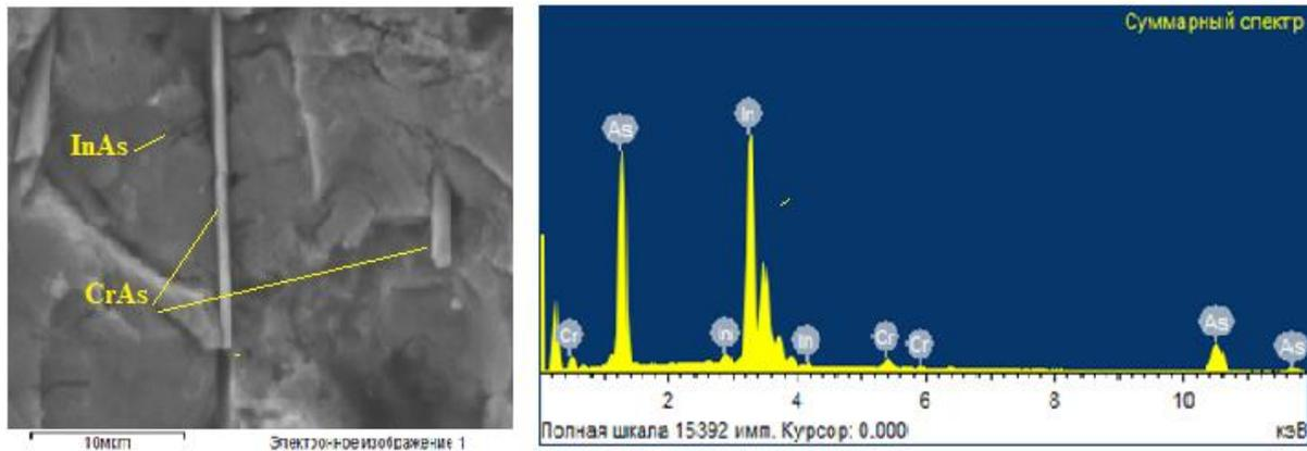
**Figure 3.** X-ray spectra of InAs-CrAs eutectic obtained with SEM–EDX from the needle and matrix phases along the lateral directions of the specimens.
