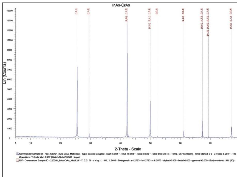
Figure 1 X-ray spectrum of InAs-CrAs eutectic composite.
