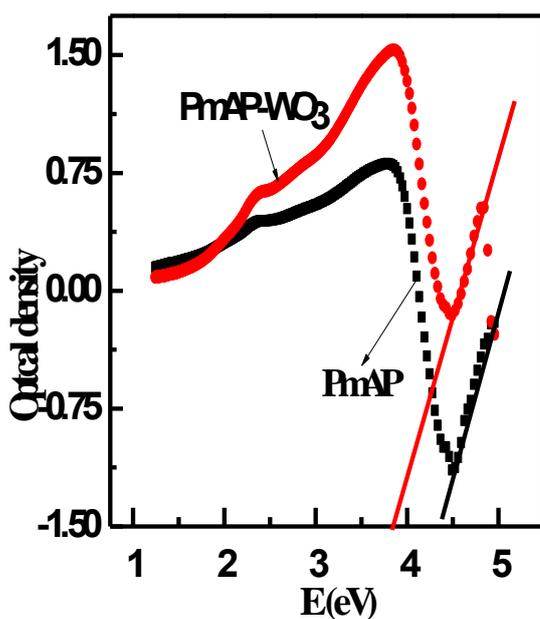
Figure 2. Band gap (right side Figure.1) of PmAP polymer and PmAP/WO<sub>3</sub> composites
