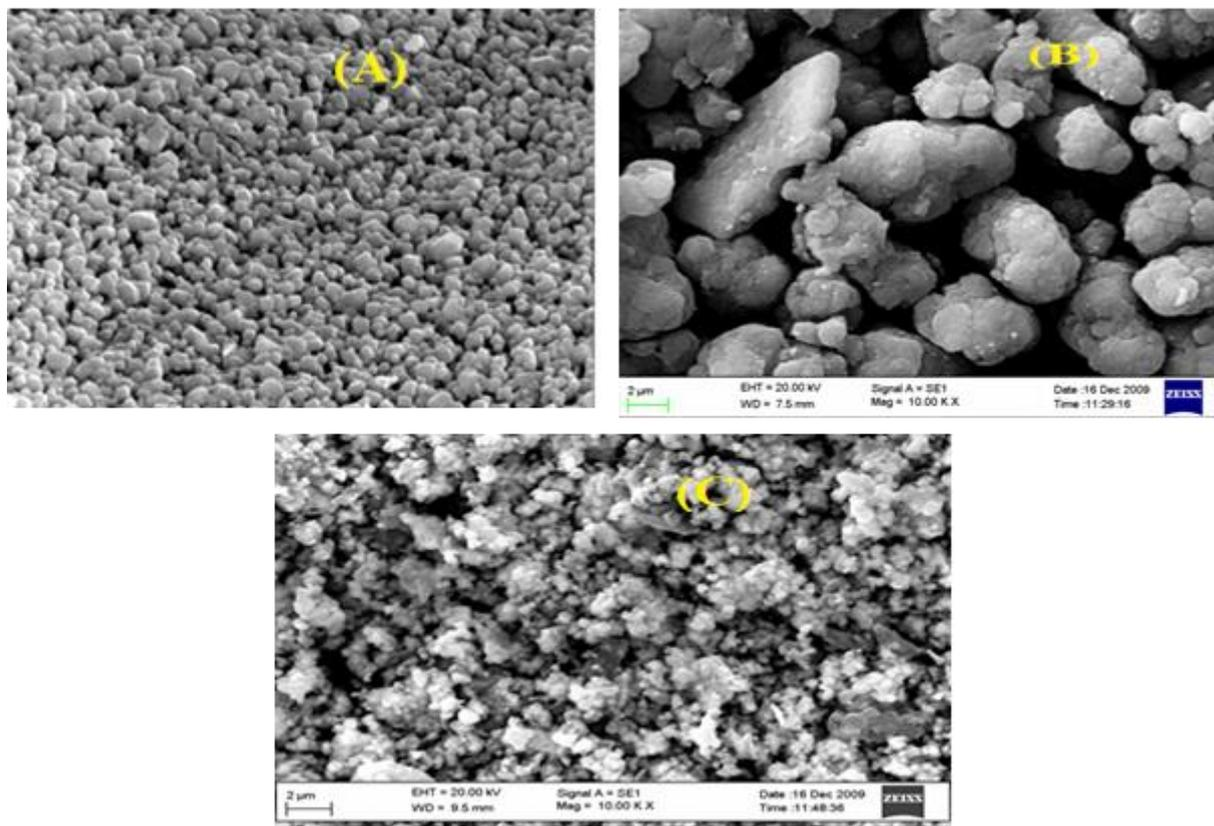
**Figure 3.** SEM images of WO<sub>3</sub> (A), PmAP (B), PmAP/WO<sub>3</sub> composite (C)
