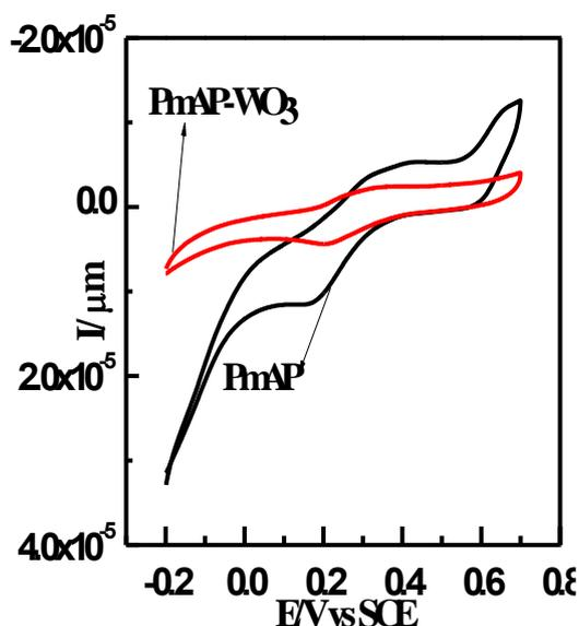
**Figure 4.** Voltammograms (CV) of PmAP and PmAP/WO<sub>3</sub> composite
