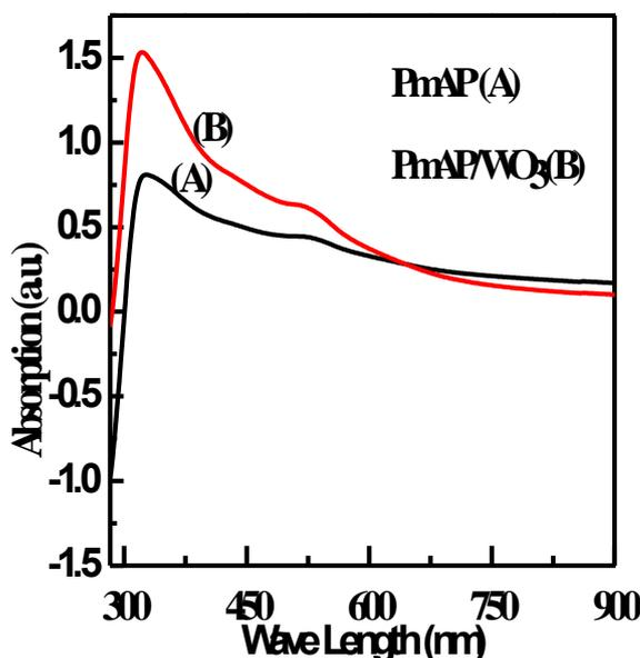
Figure 1. Superimposed UV Visible spectra of PmAP (A) and PmAP/WO<sub>3</sub> composite(B)
