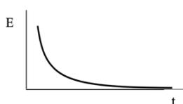
Figure 3a: Schematic diagram of the graph of Corrosion inhibition efficiency of coatings (E) against exposure time (t)
