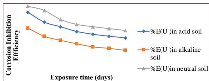
**Figure 5** Corrosion inhibition efficiency of polyurethane coated coupons in various soil media.
