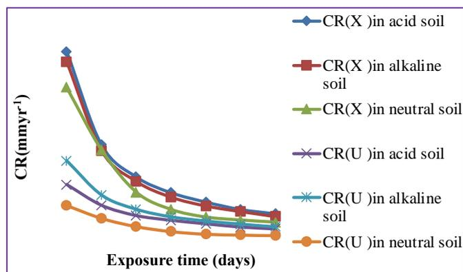
**Figure 4** Corrosion rate of coupons (uncoated and coated) in various soil media.
