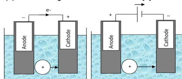
Figure 1a. Typical galvanic corrosion cell
