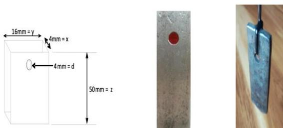
Figure 2a Shape and dimensions of the uncoated coupon      Figure 2b Uncoated coupon      Figure 2c Polyurethane coated coupon
