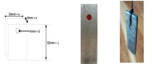
Figure 2a Shape and dimensions of the Figure 2b Uncoated Figure 2c Polyurethane uncoated coupon coupon coated coupon
