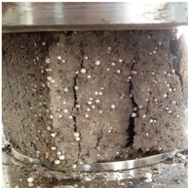
Figure 3. Failure pattern of Novel Geomaterial (NGM) specimen.
