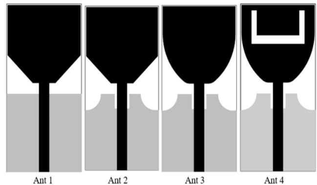
Figure 2. Evolution of antenna structure.
