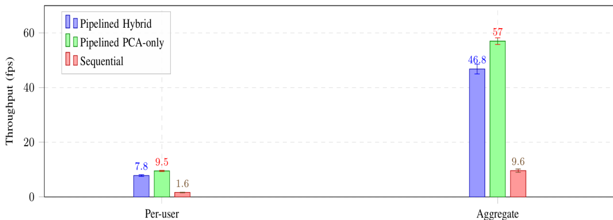
Figure 7. Aggregate throughput comparison at 6 concurrent users (error bars: \pm 1 std over 5 runs)
