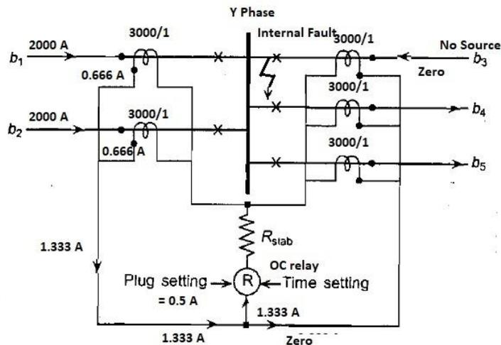
Fig3. Behaviour of busbar differential scheme on internal fault
