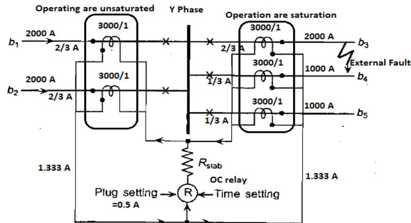
Fig4. Behaviour of busbar differential scheme on external fault
