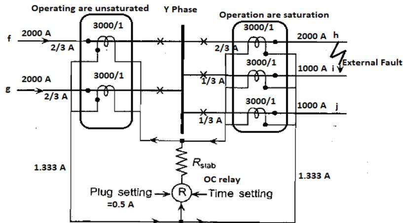
Fig5. Behaviour of busbar differential scheme on external fault
