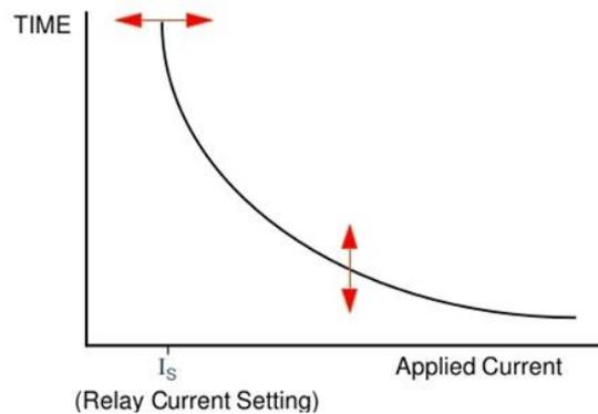
Fig2. IDMT Relay Curve
