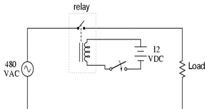
*Fig 1. Circuit Diagram of Relay*
