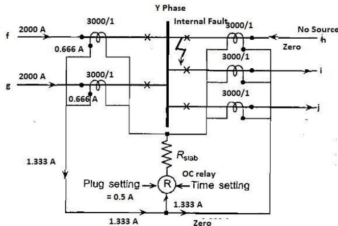
Fig6. Behaviour of busbar differential scheme on internal fault
