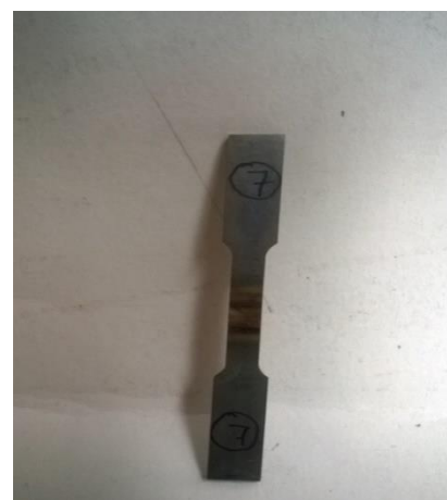
Figure 5. Photographic view of tensile sample no.7
