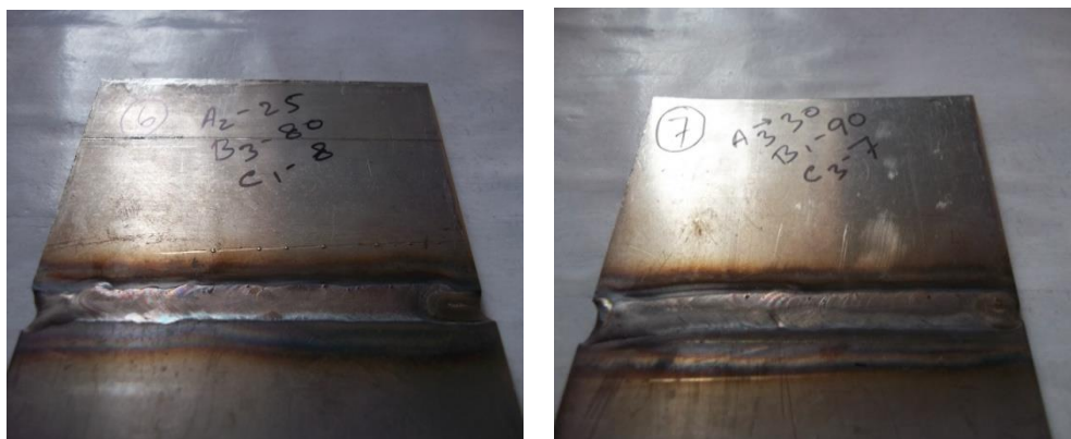
Figure 3. Photographic observation of welding sample no 6 & 7
