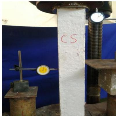
*Fig 5.2. Testing of conventional R.C column*
