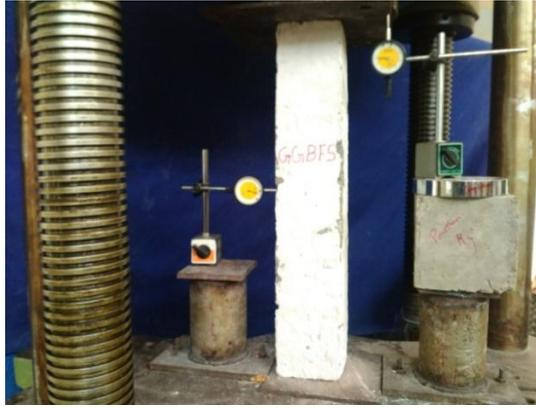
***Fig 5.3 Testing of Bacillus Bacteria Replaced R.C Column***
