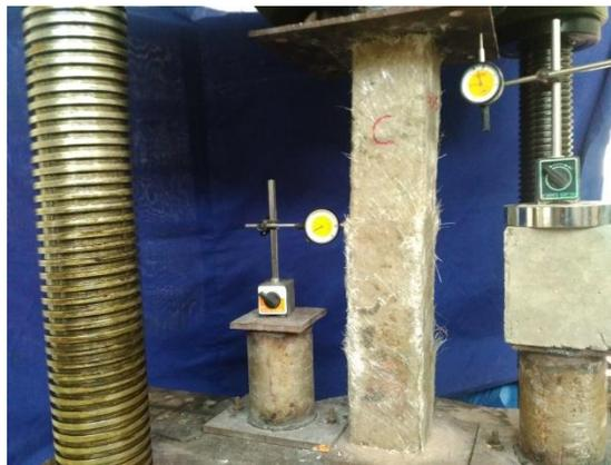
***Fig 5.5. Testing of GFRP wrapped conventional column***
