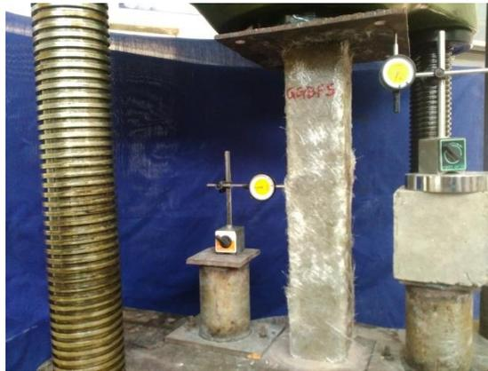
***Fig 5.4 Testing of Gfrp Wrapped Bacillus Bacteria Column***
