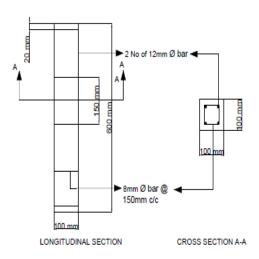
Fig.5.1. Longitudinal and cross section detailing of compressive member
