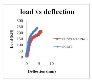
Fig.5.6. Ultimate load vs. deflection for conventional and BACILLUS Bacteria replaced columns.
