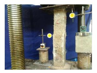
Fig 5.5. Testing of GFRP wrapped conventional column
