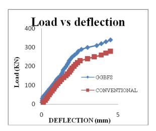
Fig. 5.7. Ultimate load vs. deflection for strengthened conventional and BACILLUS Bacteria replaced columns.
