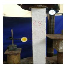
Fig 5.2. Testing of conventional R.C column
