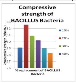
Fig 3.5. Bar diagram for compressive strength of BACILLUS Bacteria
