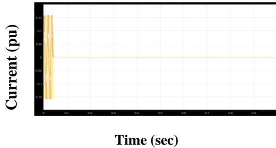
Fig 10. LLL Fault of Plot current at Bus 8
