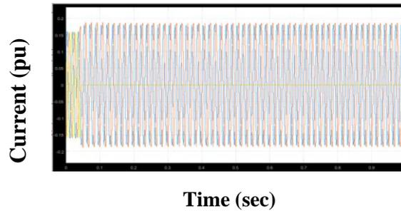
Fig 13. LG Fault of Plot current at Bus 8
