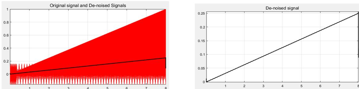
Fig 17. LL Fault at Bus 8 Original signal & De-noised Signal
