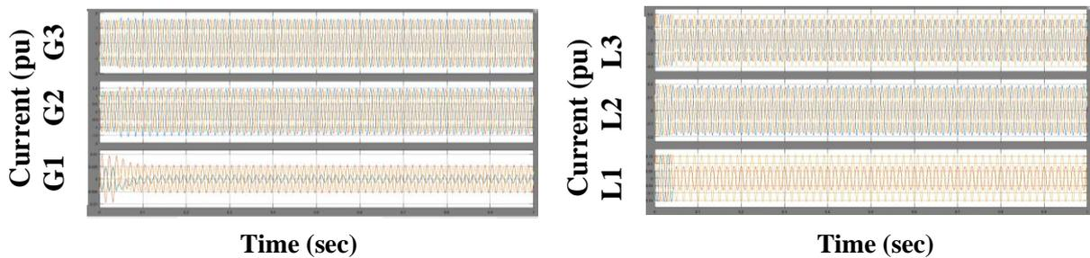
Fig 15. LL Fault at (a) Generators current & (b) Loads current
