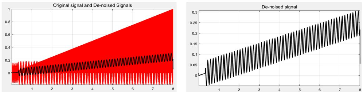
Fig 14. LG Fault at Bus 8 Original signal & De-noised Signal
