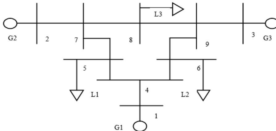
Fig 3. Single Line Diagram of IEEE 9 Bus System
