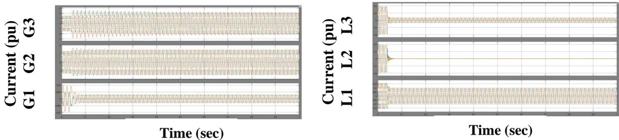
Fig 21. Internal fault at Bus 4 (a) Generators current & (b) Loads current
