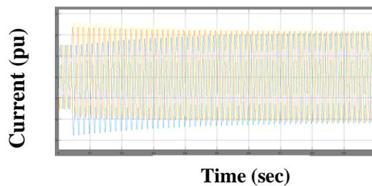
Fig 22. Internal fault of Plot current at Bus 4
