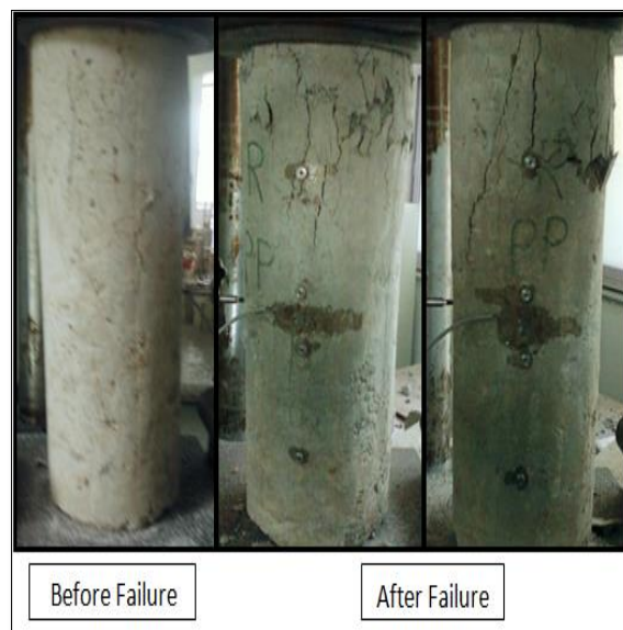
Figure 22 Crack patterns and failure mode of HPPFRC
