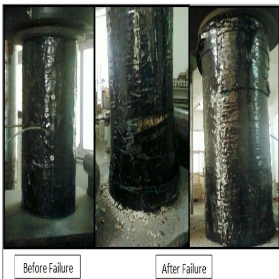
Figure 26 Crack pattern and failure mode HCWRC
