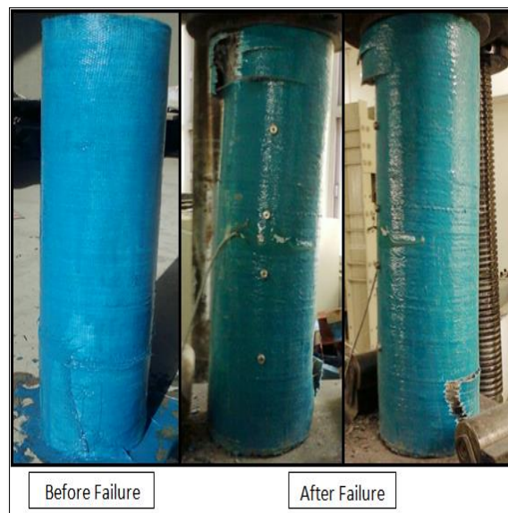
Figure 23 Crack pattern and failure mode UHWRC
