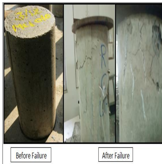
Figure 18 Crack patterns and failure mode of UHRC
