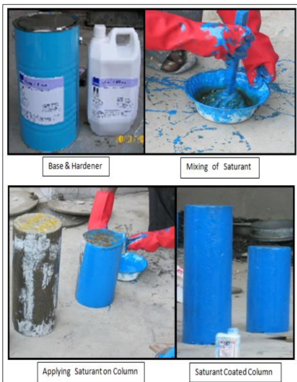
Figure 3 Application of saturant on column surface
