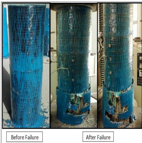
Figure 24 Crack pattern and failure mode UHCWRC
