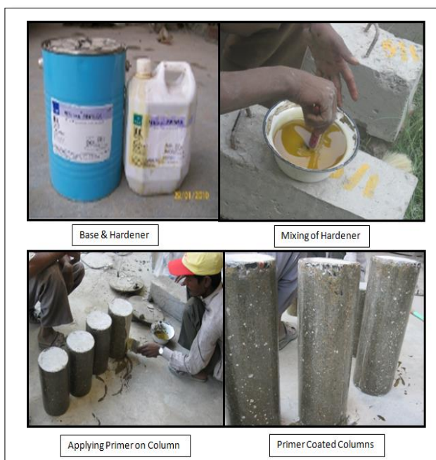
Figure 1. Application of primer on column surface.
