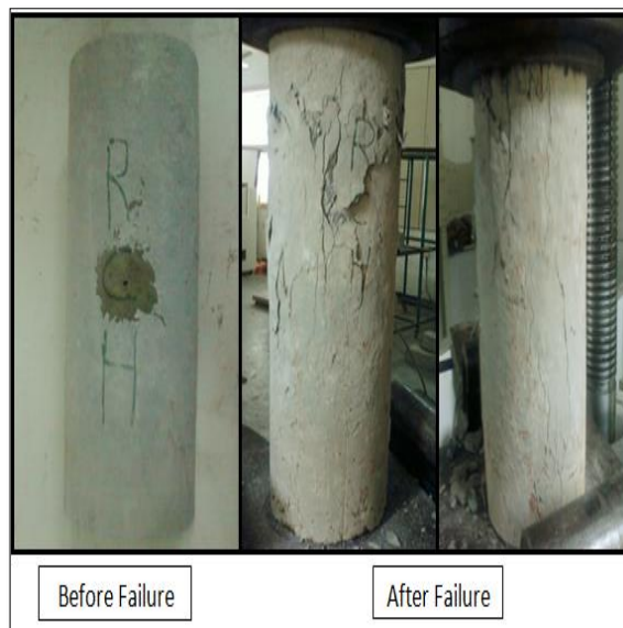
Figure 19 Crack patterns and failure mode of HRC
