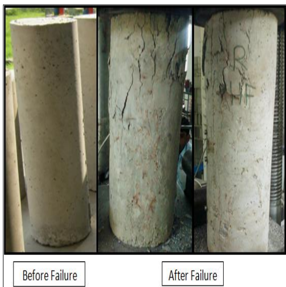
Figure 21 Crack patterns and failure mode of HHFRC
