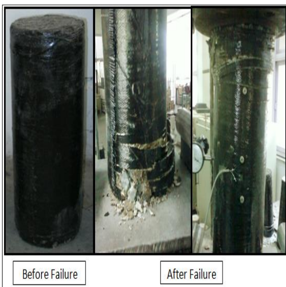
Figure 25 Crack pattern and failure mode HGWRC
