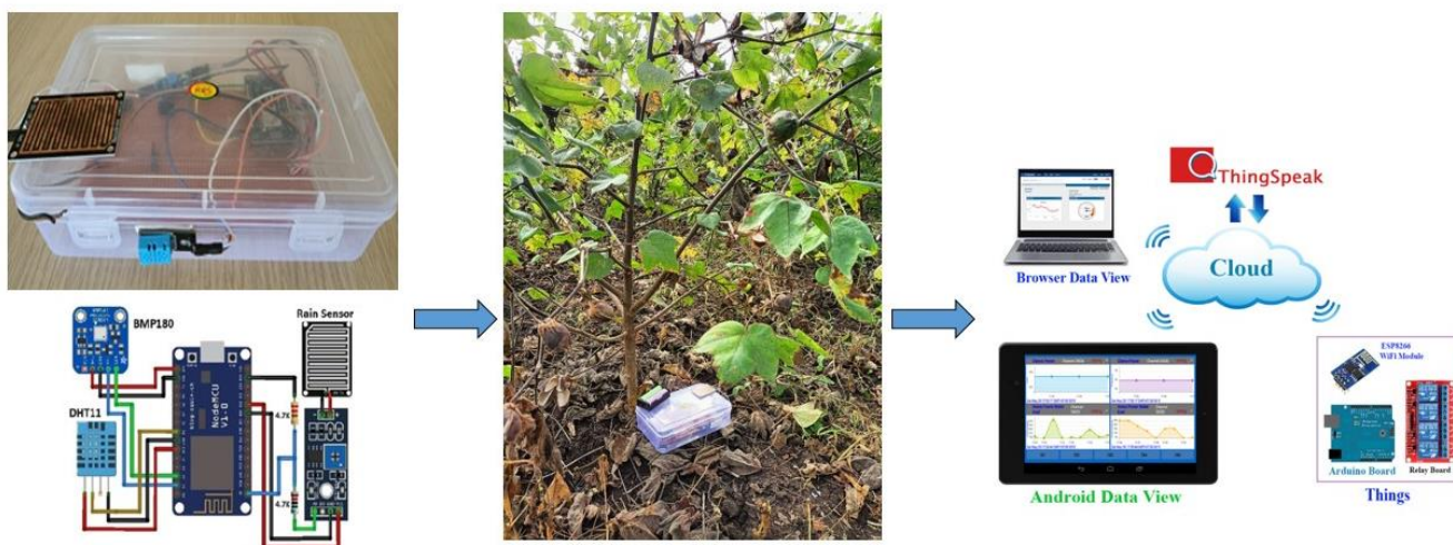
Figure 2. IoT Based System implemented on cotton field
