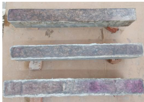
Fig 5. Beam bonded with Laminates
