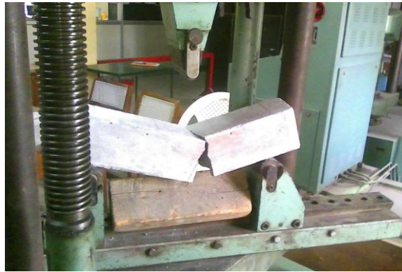
Fig 5. Flexural strength of concrete beams
