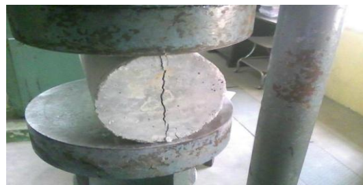
Fig 3. Split tensile strength test
