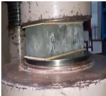
Fig 3: Compression test of Plastic Brick
