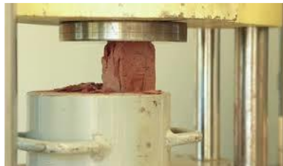
Figure 4.2 After Failure of Brick
