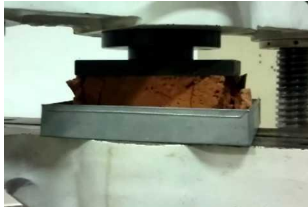
Figure 4.1 Before Failure of brick
