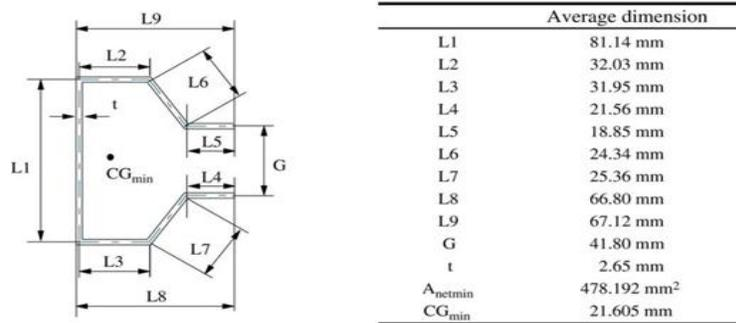
**Fig.4 Cross section of the column**
