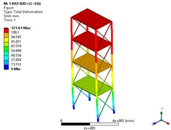
Fig. 11 Result of End Bay Deformation
