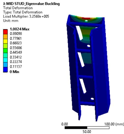
*Fig. 9 Result of Flange Warping*
