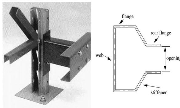
*Fig. 3 Connections in the column, “Rack” cross-section type and nomenclature.*
