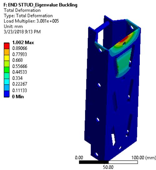
*Fig. 8 Result of Rear Flange Warping*
