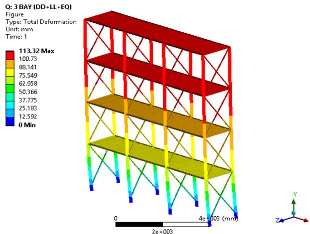
Fig. 11 Result of Mid Bay Deformation
