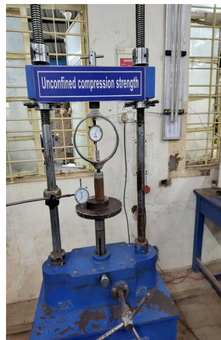
Figure 2. Testing the sample in The Unconfined Compression Strength (UCS) machine
