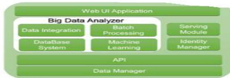
Fig 4. Cloud Computing Tier modules
