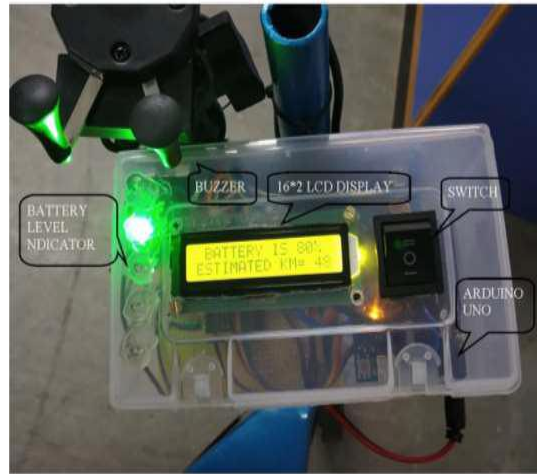
Fig. 4 Hardware Implemented Battery Level Indicator
