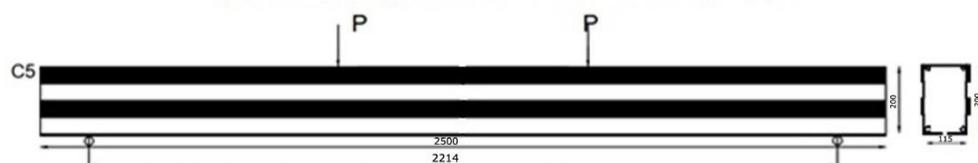
Fig.3e : Wrapping of beam along length with 50 mm spacing – C5
