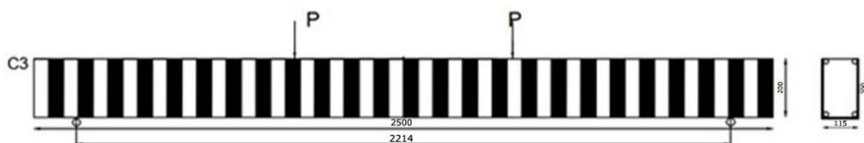
Fig.3c : Wrapping of beam at 90° with 50 mm spacing (U shaped) – C3
