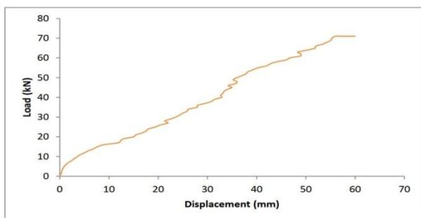
Fig. 10d : Load vs Displacement curve at centre of beam C4
