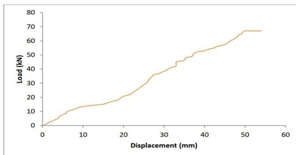
Fig. 10c : Load vs Displacement curve at centre of beam C3
