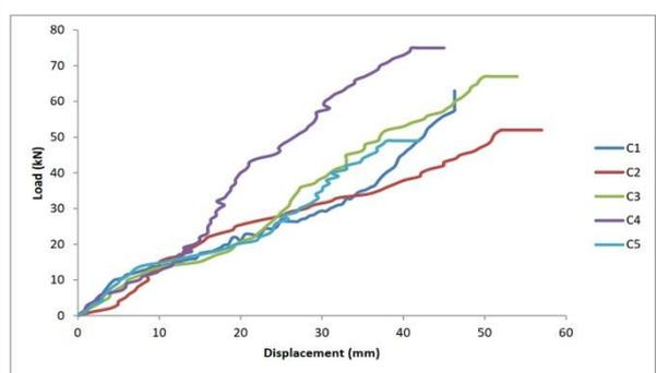
Fig. 10f : Load vs Displacement curve at centre for all cases
