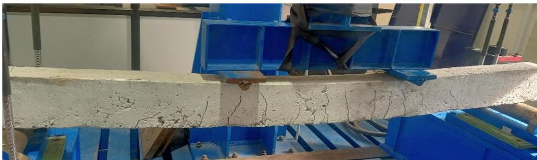
Figures 4. Mode of Failure for No wrapping (Control Beam) – C1
