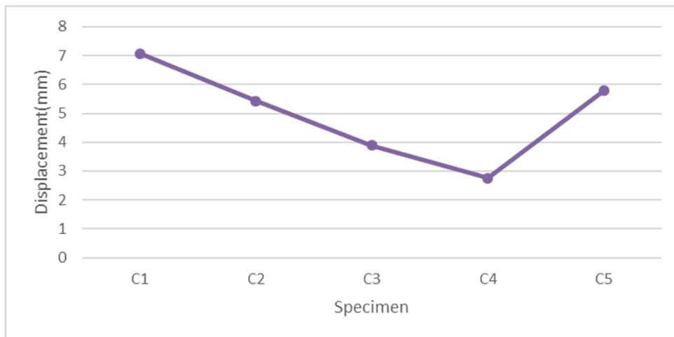
Figure 9. Displacement at Centre of beam
