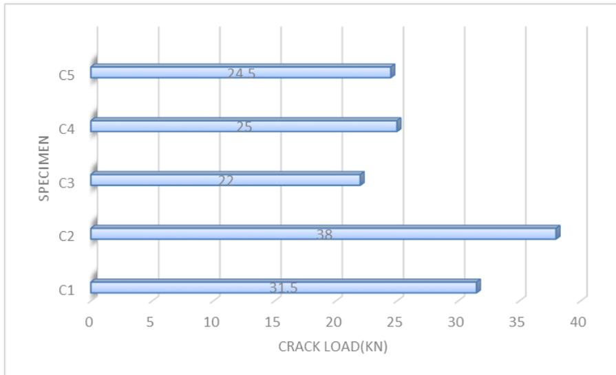
Figure 6. Initial Crack load of five different cases of beams
