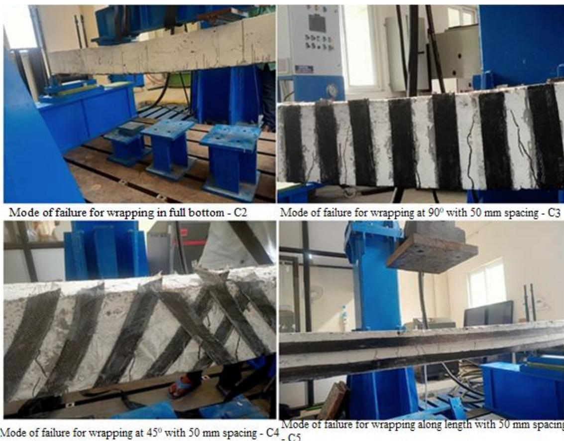
Mode of failure for wrapping in full bottom - C2      Mode of failure for wrapping at 90° with 50 mm spacing - C3
