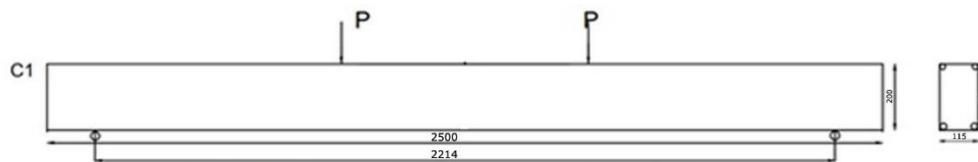
Fig.3a : Beam without wrapping (Control Beam) – C1
