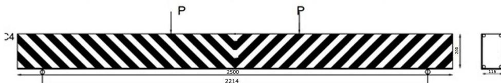
Fig.3d : Wrapping of beam at 45° with 50 mm spacing – C4
