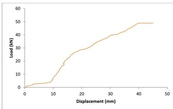
Fig. 10a : Load vs Displacement curve at centre of beam C1
