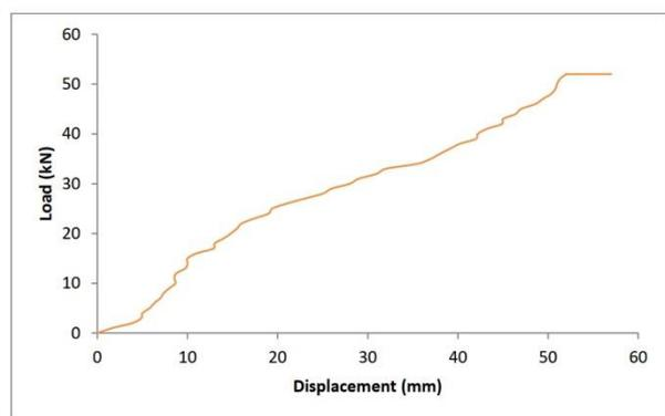
Fig. 10b : Load vs Displacement curve at centre of beam C2
