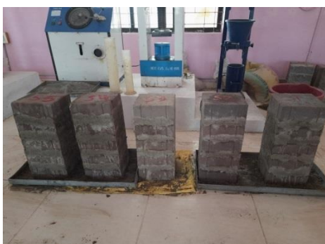
Figure 5. Casting of solid block masonry prisms
