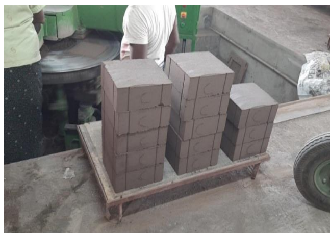
Figure 1. Casting of eco-friendly solid blocks
