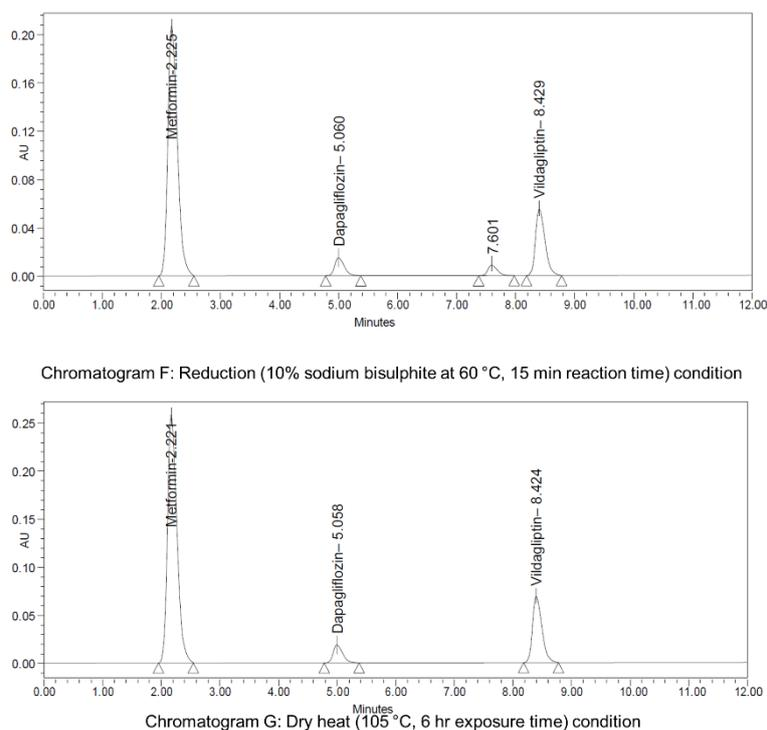
Figure 6. Chromatogram evidence for method’s specificity
