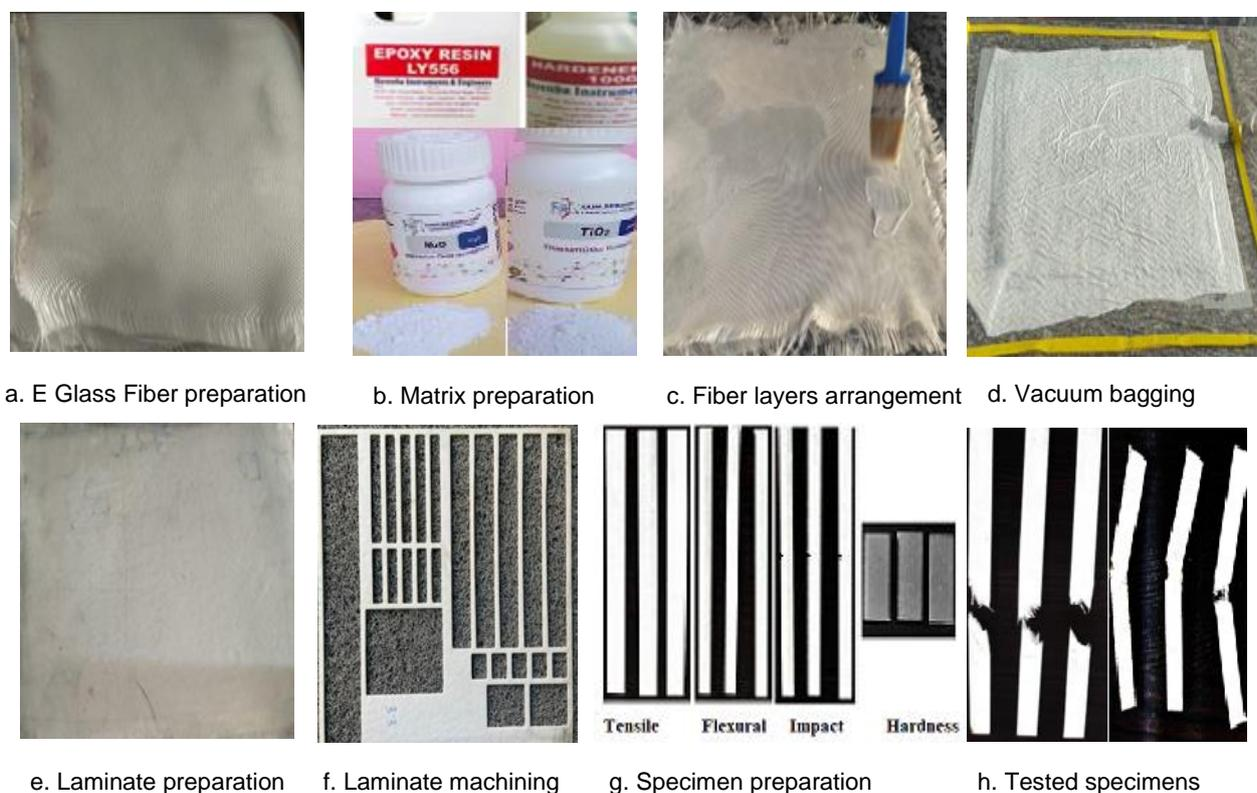
Figure 2. Procedure for creating composite samples
