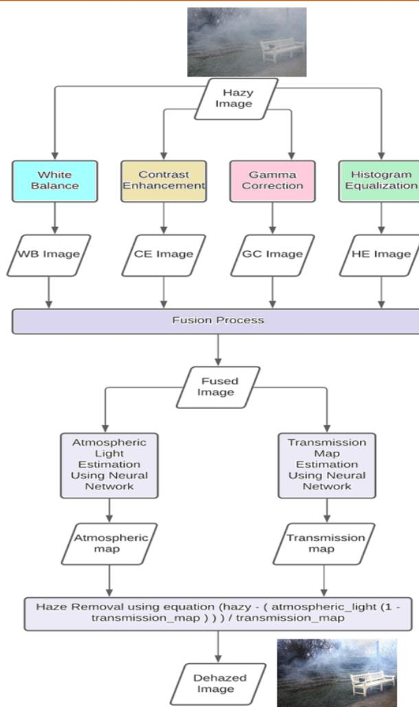
**Figure 1.** Block diagram of proposed weighted fusion of pre-processing techniques for neural network-based Image Haze Removal
