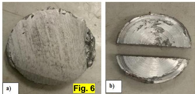
**Figure 1.** AA5052 alloy machining chips **2.** Pre-compact discs of AA5052 alloy machining chip **3.** Experimental set up for FSC process **4.** Photographs of tooling used for FSC process **5.** The DTZH pressure gauge for controlling applied force **6.** A consolidated disc specimen with a) Horizontal cross-section and b) Vertical cross
