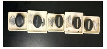
**Figure 7.** FSC disc specimens for microstructure examination.
