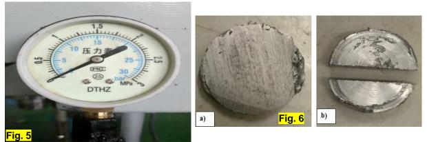
**Figure 1.** AA5052 alloy machining chips **2.** Pre-compact discs of AA5052 alloy machining chip **3**. Experimental set up for FSC process **4**. Photographs of tooling used for FSC process **5**. The DTZH pressure gauge for controlling applied force **6**. A consolidated disc specimen with a) Horizontal cross-section and b) Vertical cross
