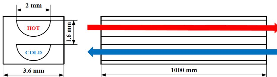
Figure 21. Physical model and geometric dimensions of a single-channel PCHE [20]
