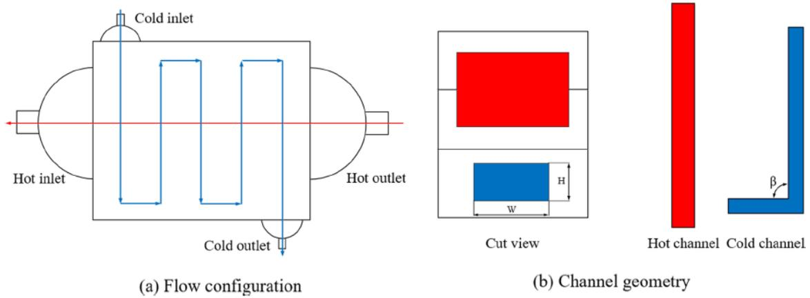
Figure 1. Flow configuration and channel geometry of designed PCHE prototype [7].
