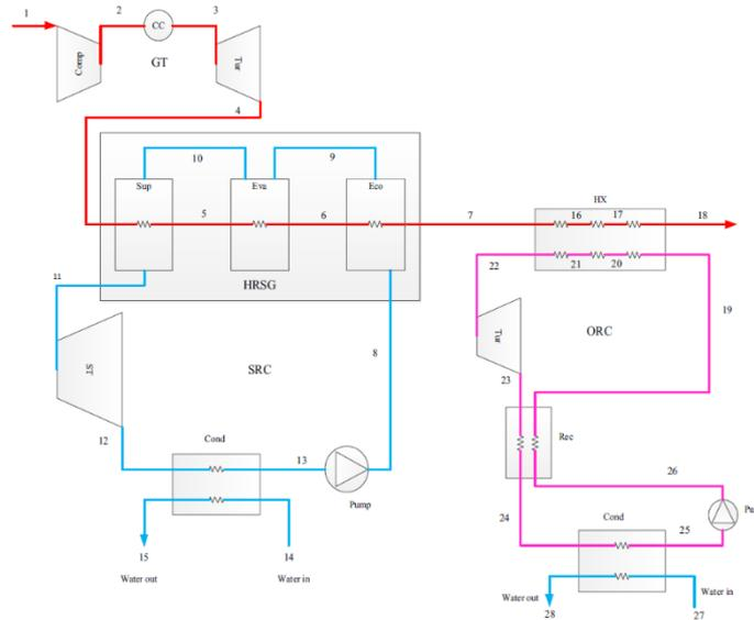
Figure 27. Proposed combined gas turbine, steam, and organic Rankine cycle [69]
