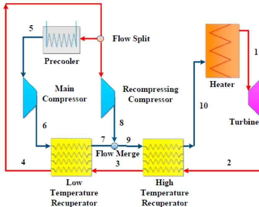
Figure 41. The configuration of the recompression cycle [78], [19]
