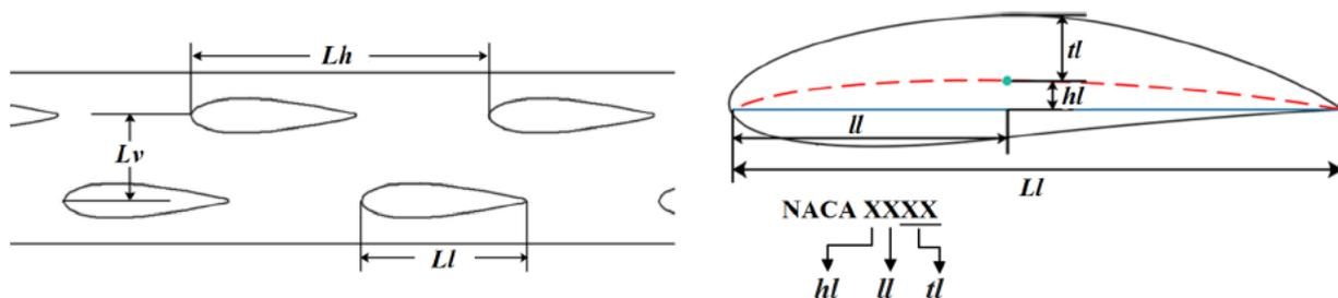
**Figure 12.** Structure and geometry parameters of PCHE channel with NACA (National Advisory Committee for Aeronautics) airfoil fins [Airfoil fin structure parameters (arc height  $h_l$ , maximum arc height position  $l_l$ , airfoil thickness  $t_l$ ), Airfoil fin arrangement parameters (airfoil fin horizontal spacing  $L_h$  and airfoil fin vertical spacing  $L_v$ ), Airfoil chord  $L_l$ ] [11]
