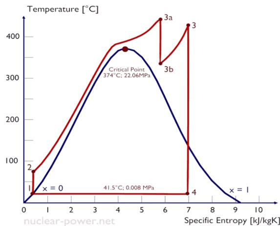
Figure 39. Process diagram for Supercritical Rankine cycle with reheat [74]
