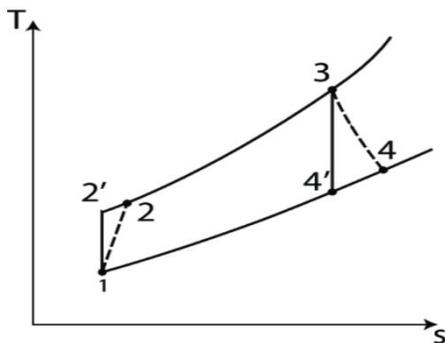
Figure 24. Process diagrams for the Brayton cycle [60]
