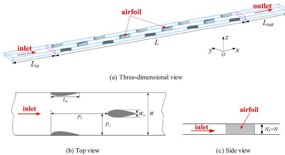
Figure 19. Schematic diagram of the physical model [17]
