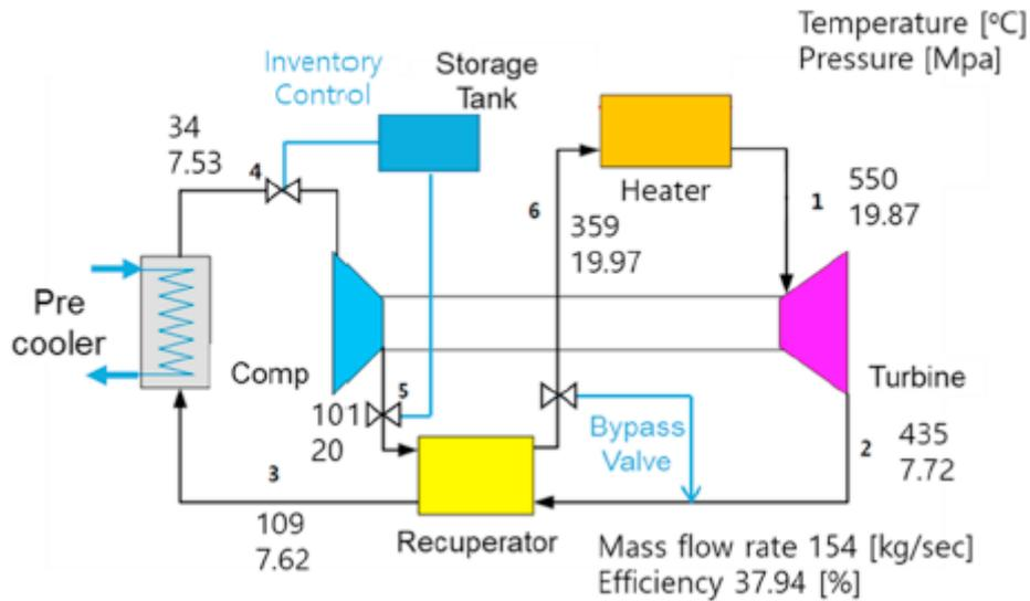
Figure 40. The configuration of the simple recuperated cycle [19]
