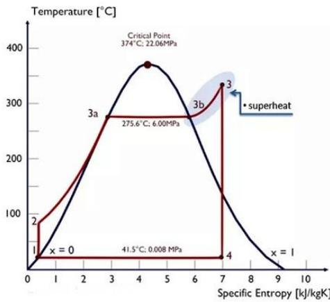
**Figure 32.** Rankine cycle with superheat of saturated steam [62]
