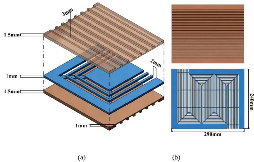
Figure 4. Improved structure: rectangular and hollow channel plate structure [7]
