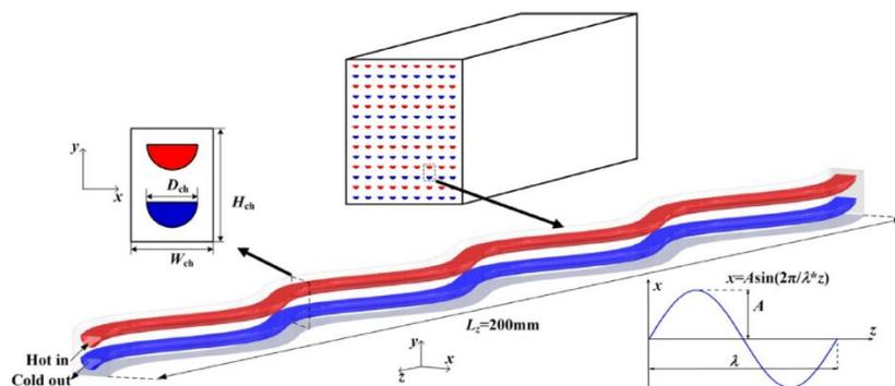
Figure 17. Geometry of the wavy channel [16]
