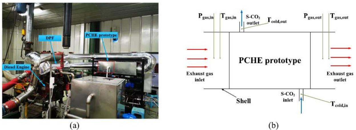
Figure 3. The experimental bench of PCHE prototype (a) and distribution of measurement points of PCHE prototype (b) [7]
