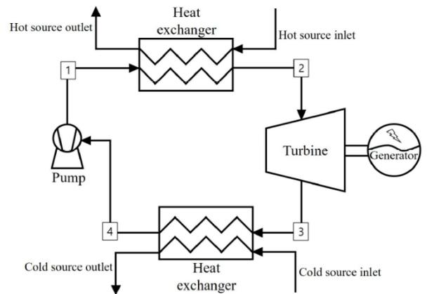
Figure 25. A schematic diagram of a simple Rankine cycle, showing the correct location of the components and the correct direction of energy and mass flows [61], [62]
