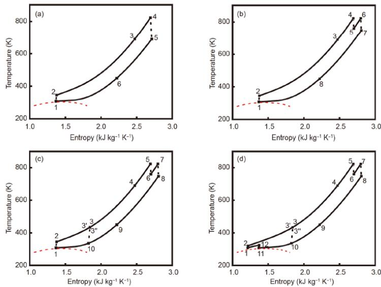
**Figure 31.** (Color online) T-s diagrams of (a) simple recuperative cycle, (b) reheating cycle, (c) recompression cycle, and (d) intercooling cycle [60]
