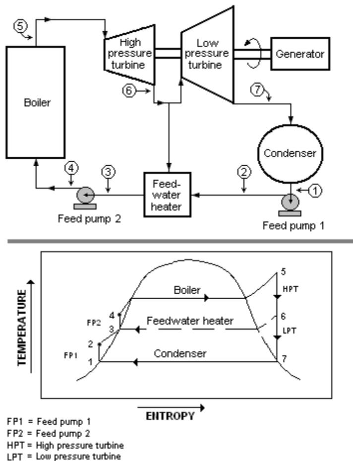
Figure 38. A Rankine cycle with two pumps, two steam turbines and a single open feedwater heater [73]; [62]
