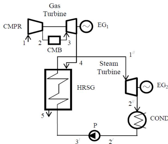
CMPR – air compressor; CMB – combustor; EG<sub>1</sub> – gas turbine electric generator; HRSG – heat recovery steam generator; EG<sub>2</sub> – steam turbine electric generator; COND – condenser; P – pump
