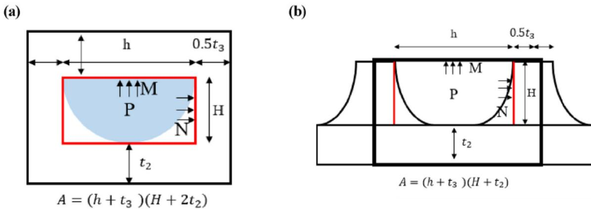
Figure 5. Geometry of PCHE: (a) Straight, zigzag, and wavy types; (b) airfoil type [8]
