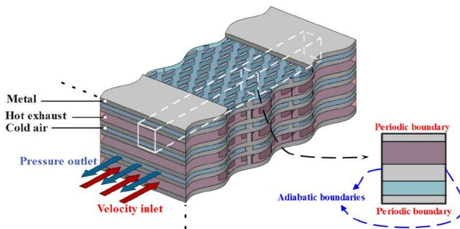
Figure 11. Computational domain and boundary conditions of PCHE [11]
