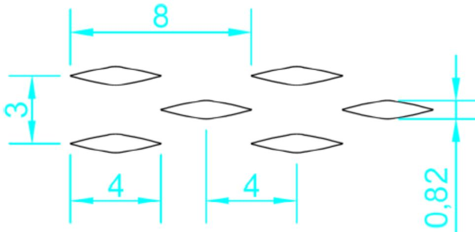
Figure 7. Geometric size of rhombic fin arrangement [9]
