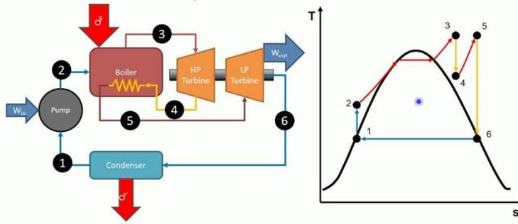
Figure 34. Rankine cycle with reheat of superheated steam [74]
