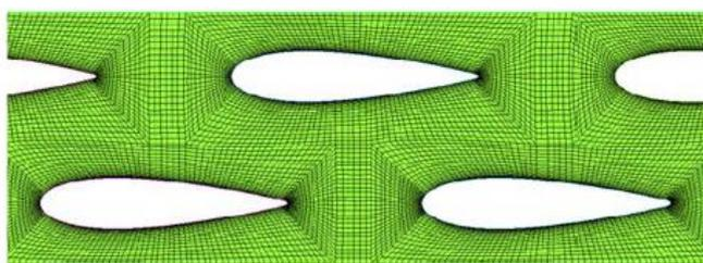
**Figure 13.** Computational grids of AF-PCHE channel [11]
