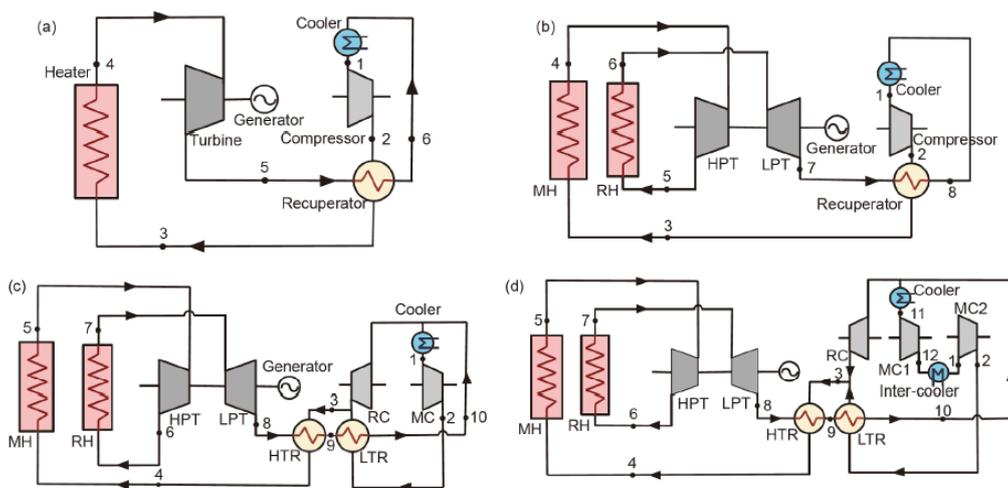
**Figure 30.** Configurations of (a) simple recuperative cycle, (b) reheating cycle, (c) recompression cycle, and (d) intercooling cycle. MH: main heater, RH: re-heater, HPT: high-pressure turbine, LPT: low-pressure turbine, MC: main compressor, RC: re-compressor, HTR: high-temperature recuperator, LTR: low-temperature recuperator [60]
