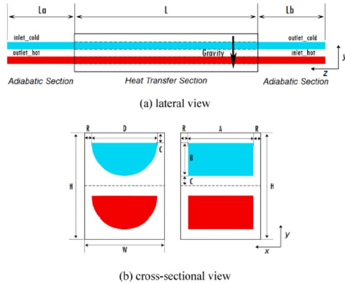
Figure 10. Physical model geometry of calculation unit [10]
