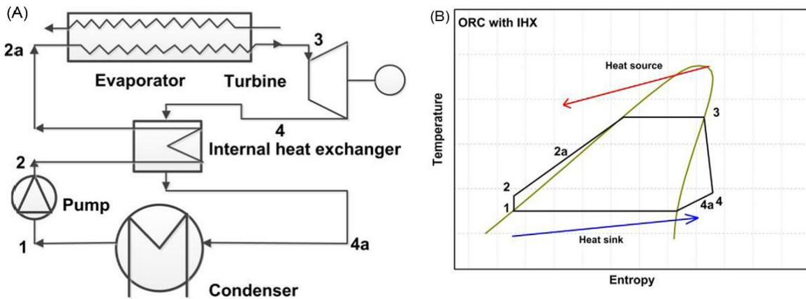
Figure 36. Schematics of a reheat ORC system: (A) system schematic and (B) T-S diagram [71]
