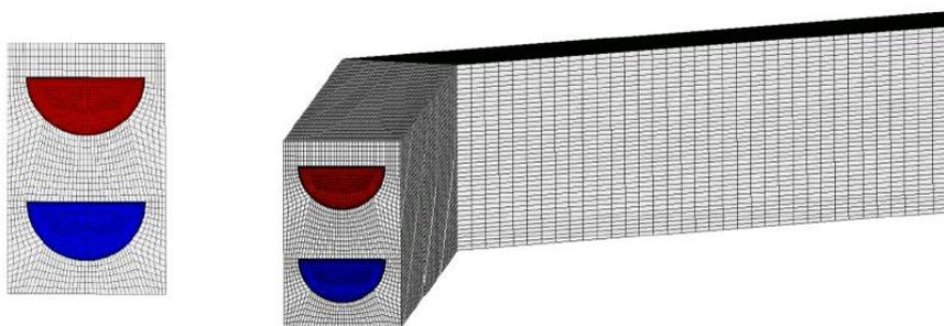
(b) Meshing model of the geometrical model
