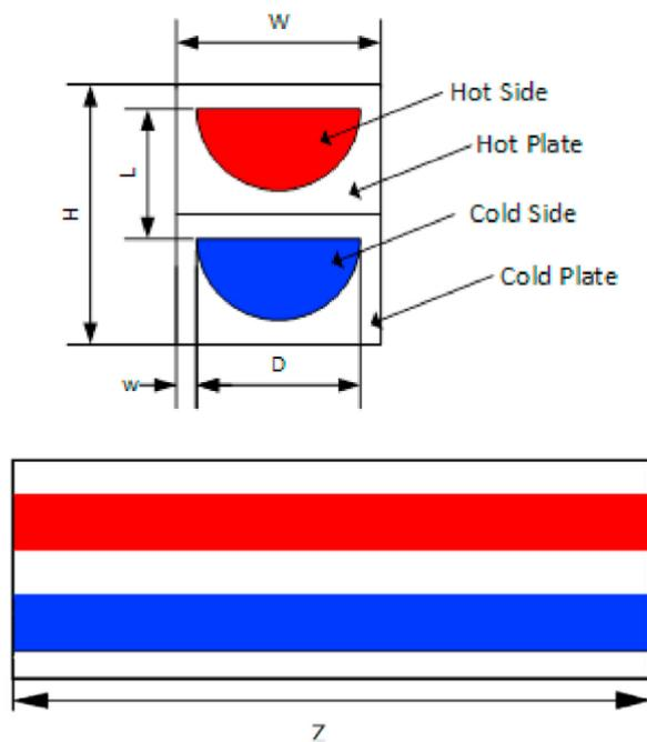
Figure 16. Geometry and dimensions of PCHE [14]
