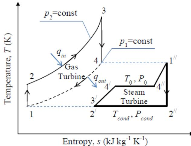
1–2–3–4 is the idealized Brayton cycle; 1''–2''–2'–3'–4'–4'' is the idealized Rankine cycle;  $q_{in}$  and  $q_{out}$  are the heat supplied to and removed from the exhaust gases in the isobaric process at pressures  $p_2$  and  $p_1$ , respectively
