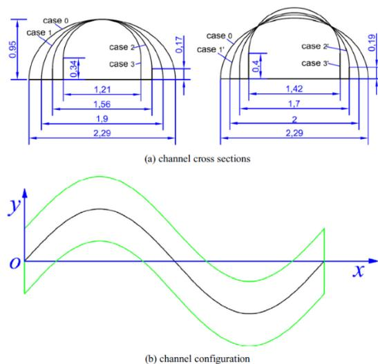
Figure 22. Shapes and sizes of the PCHE channel (unit: mm) [21]
