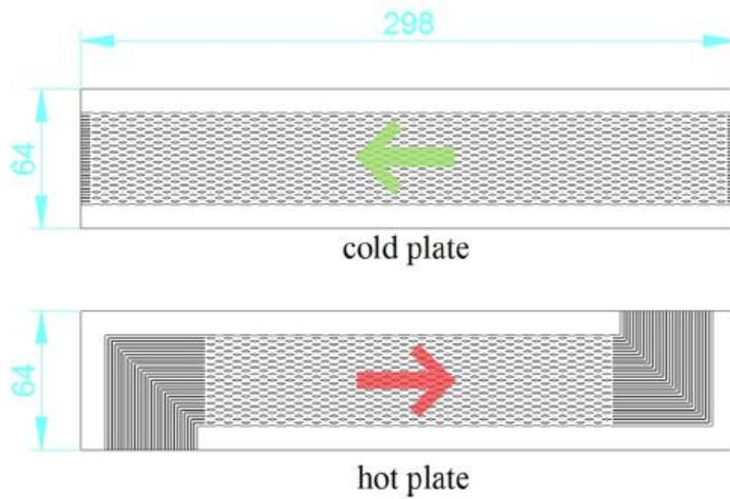
Figure 8. Geometry of the rhombic fin channels [9]
