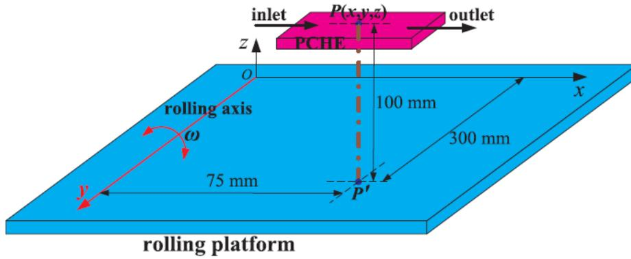
Figure 18. Schematic diagram of the rolling working condition [17]
