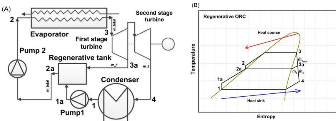
Figure 37. Schematics of a regenerative ORC system with recompression (two pumps): (A) system schematic and (B) T-S diagram [71]
