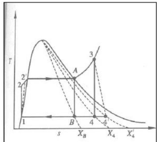
Figure 26. Temperature–entropy process diagram for a basic binary cycle using a working fluid with normal condensing properties [61], [62]
