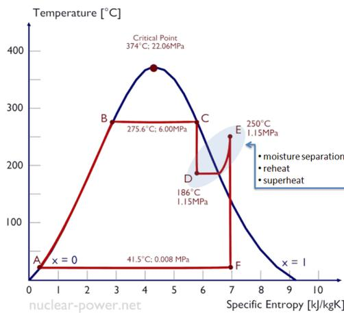
**Figure 33.** Rankine cycle with reheat of wet steam and superheat of saturated steam [61], [62]
