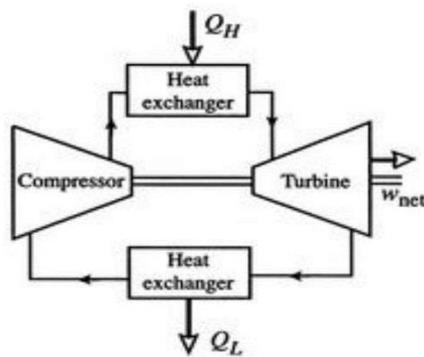
Figure 23. Closed-cycle system (Liu *et al.* [60]).
