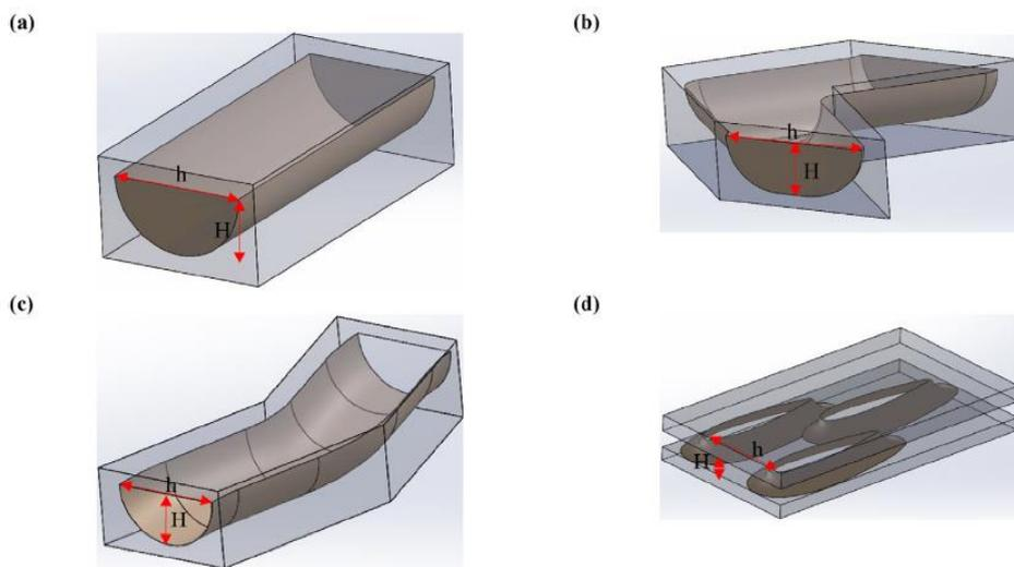
Figure 6. Three-dimensional channel types: (a) Straight; (b) zigzag; (c) wavy; (d) airfoil [8]
