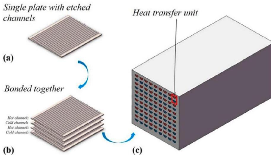
Figure 9. Heat transfer unit structure of PCHE with straight channels [10], [22]
