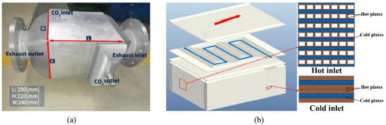
Figure 2. The photograph and geometric structure of PCHE prototype [7].
