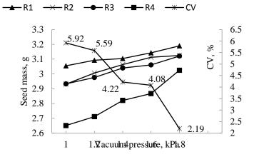
Figure 3c. Results of 30° vacuum opening angle on rows seed pick-up at 15 r.min<sup>-1</sup>.
