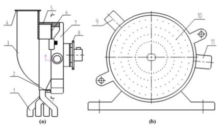
Seed tubes; 2. Seed discharge nut; 3. Seed box; 4. Seed box cover; 5. Metering plate shield; 6. Metering plate 7. Pressure chamber; 8. Driving sprocket; 9. Vacuum inlet; 10. Metering plate nozzles;
