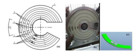
Vacuum distributor body; 2. Separators; 3. Vacuum openings; 4. Movable opening covers; 5. Protrusion on the covers for easy dragging.
