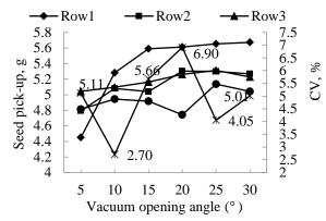
Figure 4e. Results of opening angles on rows picking performance at 25r.min<sup>-1</sup> and 1.8 kPa.
