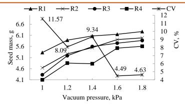
Figure 3f. Results of 30° vacuum opening angle on rows seed pick-up at 30 r.min<sup>-1</sup>
