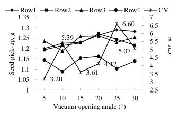
Figure 4 a. Results of opening angle on rows picking performance at 5 r.min<sup>-1</sup> and 1kPa.
