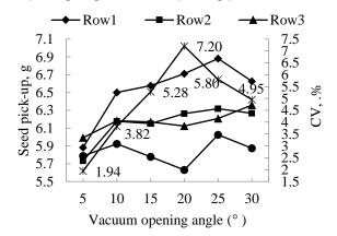
Figure 4f. Results of opening angles on rows picking performance at 30r.min<sup>-1</sup> and 1.8 kPa.
