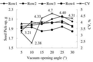
Figure 4b. Results of opening angles on rows picking performance at 10 r.min<sup>-1</sup> and 1.2 kPa
