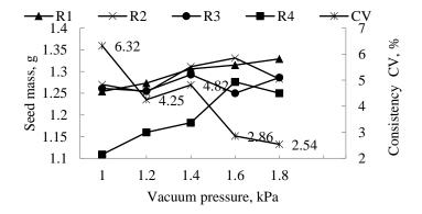
Figure 3a. Results of 30° vacuum opening angle on rows seed pick-up at 5 r.min<sup>-1</sup>.
