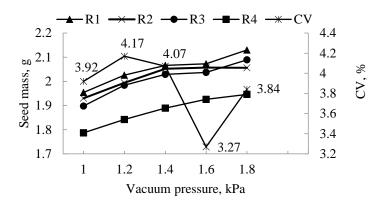
Figure 3b. Results of 30° vacuum opening angle on rows seed pick-up at 10 r.min<sup>-1</sup>.
