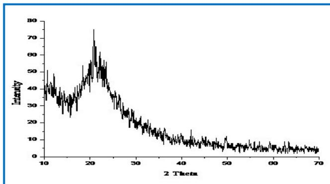
**Figure 6. XRD pattern of silica nano particles**
