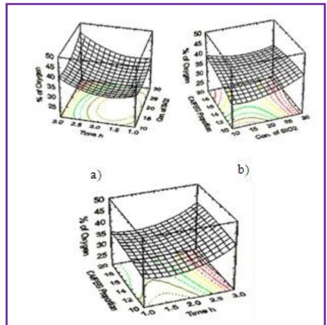
Figure 11 (a), (b) & (c) Effect of process variable on oxygen purity
