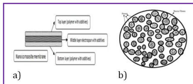
**Figure 3. a) Principle of membrane construction b) cross section of the membrane**
