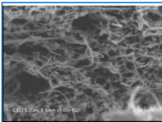
Figure 9. SEM image of the cross section of the polymeric multi layer nano composite membrane
