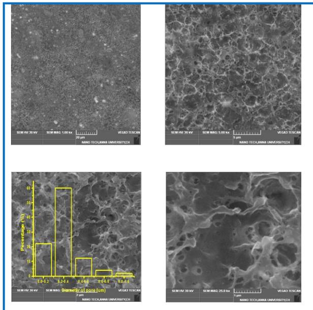
Figure 8. SEM Images of polymeric multi layer nanocomposite membrane
