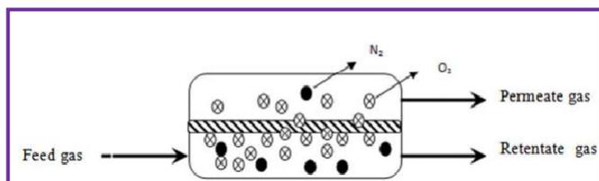
**Figure 1.** Schematic diagram of the principle of membrane gas separation process
