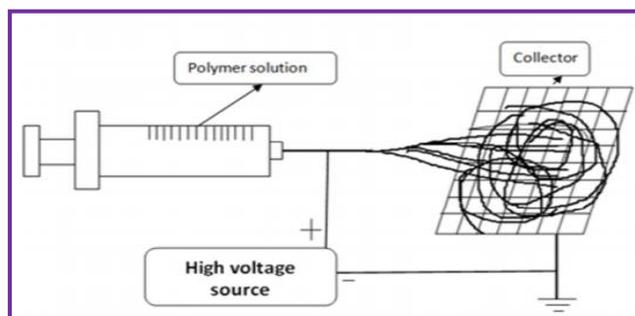
**Figure 2.** The principle of electrospinning apparatus
