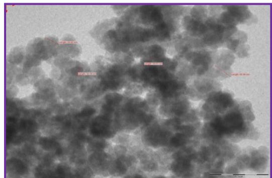
**Figure 5. TEM image of silica nano particles**
