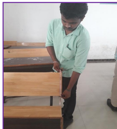
Fig 4.2 Measuring Back Rest Height
