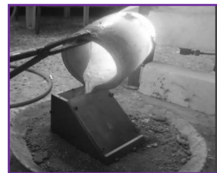
Figure 2. Pouring mixture MMCs in wedge shaped die.
